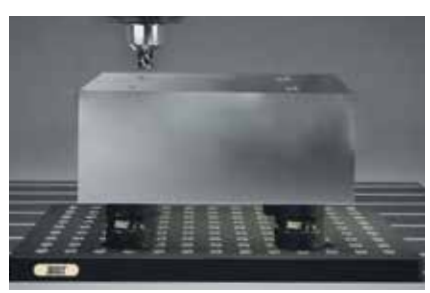
1 : MACHINING COUNTERBORES (SMALLER Ø)
